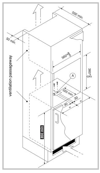
The appliance needs sufficient ventilation. Make an opening in the plinth at least 280 cm2 large for this purpose.
